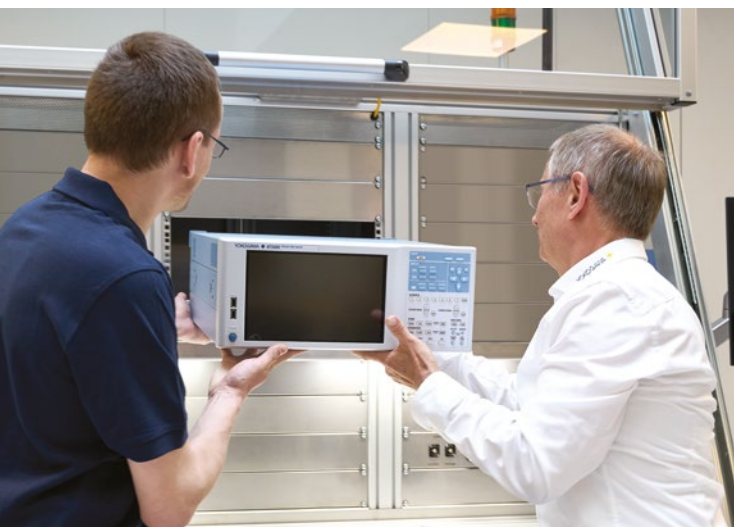
Image 1: The SAXOGY SHL safety measurement station, or Safety Housing Lab, has a modular design and can be equipped with a wide range of measurement technology.
